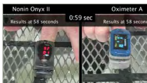
Figure 3: Nonin Onyx keeps reading while passing the 10 minute IPX2 moisture exposure test. Oximeter A stopped reading at 58 seconds. 7
