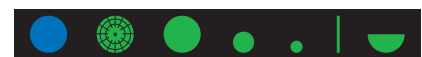
With red-free filter: Cobalt blue filter, fixation star with polar coordinates, large spot, small spot, pinhole, slit, hemislot
