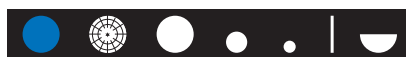
Cobalt blue filter, fixation star with polar coordinates, large spot, small spot, pinhole, slit, hemislot
