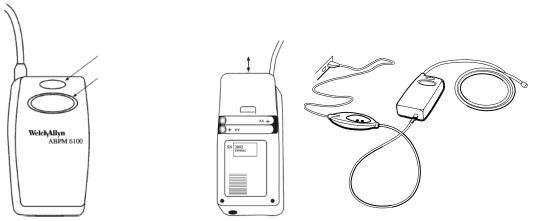
The ABPM 6100 features a simple design. One Start/Stop button functions as the primary control. The LCD (liquid crystal display) displays easy-to-read information. The CardioPerfect Workstation Software allows you to program the unit before the study and retrieve data after the study. A single air hose connector allows you to connect the cuff to the unit.
