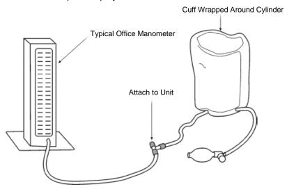
Note: Your ability to measure the accuracy of the ABPM 6100 depends upon the sensitivity of the pressure standard you use for the calibration procedure.
