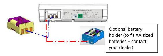
4. Place the housing back in the back of the indicator, and close the battery housing cover.
