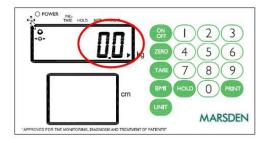
The scale will now go into weighing mode and should show 0.0kg on the display.
