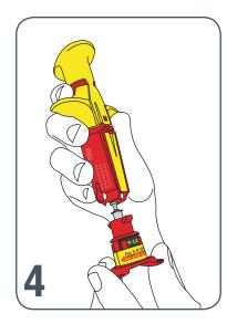
Remove NIO-SIM-P from reloading base and connect stabilizer base to device.
