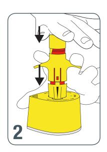
Push down on device until completely compressed onto the reloading base. While maintaining downward pressure, use other hand to push trigger wings down until a "click" is heard.
