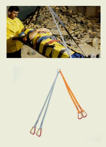
The Paraguard 4-pont lifting sling is designed for use with Paraguard rescue stretcher, tested and certificated for horizontal lifts up to the maximum SWL of Paraguard stretcher, load tested and rated up to 226 kgs. Incorporating metal carabiners that quickly attach to the 4 lifting points on the Paraguard stretcher, the Paraguard 4-point lifting sling is easy to deploy, giving Paraguard additional capability in various environments.
