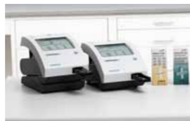
Figure 2: CLINITEK Status family of analyzers employs an algorithm for humidity-compromised reagent strip detection that helps ensure quality results.
