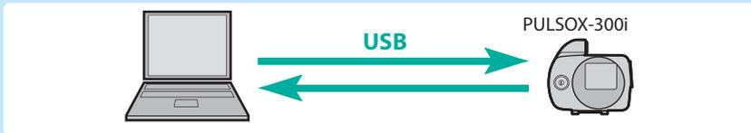
\*The above functions are available on the PULSOX-300i only. To use these functions with the PULSOX-3, it must be connected through the IF-3 interface unit and RS-232C serial port.
