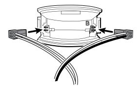
Snap the handle cradle assembly into the front housing. Make sure that the cradle assembly tab and the beveled edge are at the top of the housing.
