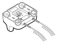
Lift and remove the rear housing.
