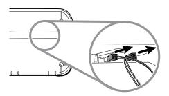
Push in the snap tabs and then remove the cradle assembly by pushing outward.
