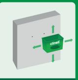
The position may change slightly in order to pick up previous fixing to avoid any more holes in the walls and hide existing holes in the wall behind the dispenser. This may result in screws that are longer or heavier gauge based on what was placed in the wall previously.
