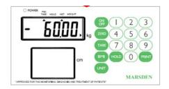
Press the ZERO key to return to normal weighing mode.
