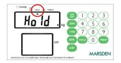
Push the bed onto the pads. The weight will hold on the screen, even if the patient moves.
