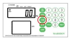
Press the TARE key for three seconds to enter Preset Tare setting mode.
