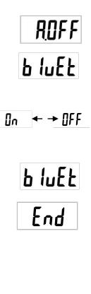
Long press the ZERO key for three seconds to enter the Setting mode and then display the A-OFF menu.
